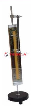
55804 Experimental Set-Up has been designed specifically verification of Hook's Law.
