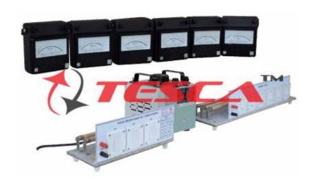
55811 Experimental Set-Up has been designed specifically to study the measure of power in a single phase circuit using (i) Three-voltmeter method. (ii) Three-Ammeter method. The set-up consists of Voltmeter, Ammeter, Variac, Fixed resistance in three steps and Variable load.
