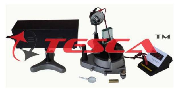
55812 Experimental Set-Up has been designed specifically to study the Polarisation of Light by Simple reflection using Laser. The set-up consists of Circular table, Diode Laser, Glass Slab, Analyser attachment with Laser Detector, Nanoammeter, Reading lens and Spirit Level.
