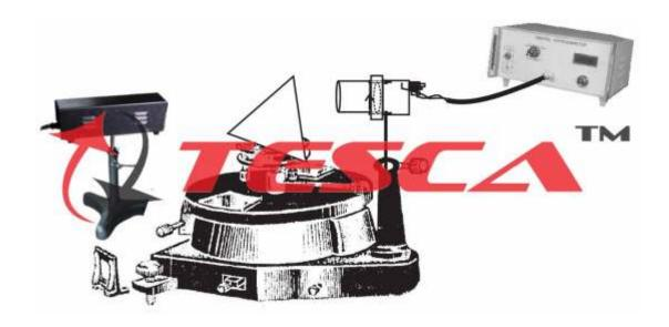
55813 Experimental Set-Up has been designed specifically to determine Brewster's angle for a glass prism surface and hence to determine refractive index of glass using Laser. The set-up consists of Circular table, Diode Laser, Glass prism, Laser Detector, Nano-ammeter, Reading Lens and Spirit Level.
