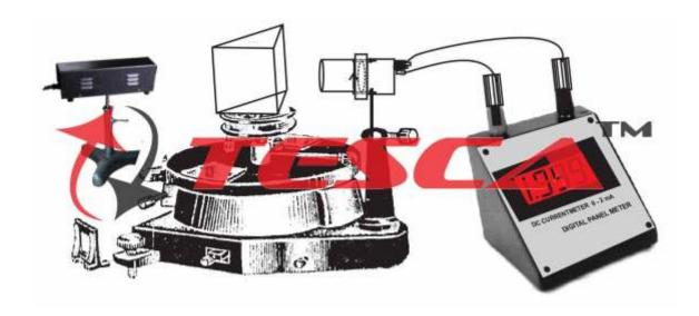
55814 Experimental Set-Up has been designed specifically to determine the Refractive Index of liquids (Water, Paraffin Oil, Glycerol, Kerosene, Benzene etc.) in the form of prism by using Laser and it's detector. The set-up consists of Circular table, Helium Laser, Hollow Prism, Laser Detector, Digital Milliammeter, Reading lens and Spirit Level.
