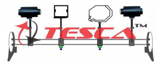
55829 Experimental Set-Up has been designed specifically to compare the illuminating power of two given source of light with a Lummer Brodhum (L.B.) Photometer. The Set-up consists of Lummer-Brodhum (L.B.) Photometer, Optical Bench & two sources of light and one ground glass plate.
