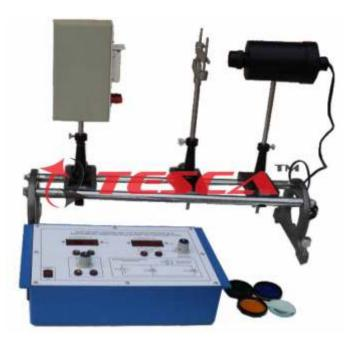
55838 Experimental setup has been designed specifically to Determine the Electronic Charge and the Work Function f a Photo Metal Using Photo Electric Cell (Vacuum Type) The experimental set-up is absolutely self contained and requires no other apparatus.
