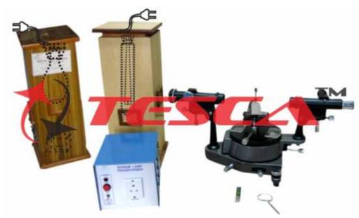
55844 Experimental Set Up has been designed specifically to calibrate the spectrometer by Mercury Vapour Lamp and hence to find the wavelength of a given monochromatic source of sodium light. The set-up consists of Spectrometer, Prism, Mercury vapour lamp, Sodium light source, Reading lens, Spirit Level etc.
