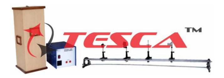
55852 Experimental Set-Up has been designed specifically to determine the Wave Length of Sodium Light Using Lioyd's Mirror. The set-up consist of Optical bench, Lioyd's Mirror, Lens Holder, Micrometer eye-piece, Optical Slit, Double Convex Lense, SOdium Light source etc.
