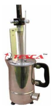
55885 Experimental Set Up has been designed specifically for to determine temperature co-efficient of resistance of metal (conductor using platinum resistance thermometer) The set up is absolutely self contained and requires no other apparatus.
