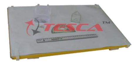
**55901** Experimental Set-up has been designed specifically to determine the refractive index (μ) of the glass prism & to study the variation of the angle of deviation with the angle of incidence using a glass prism and to determine the angle of minimum deviation Draw necessary graph for it.
