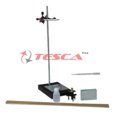
55906 Experimental Set Up has been designed specifically for finding the refractive index of a liquid by using convex lens and plane mirror.
