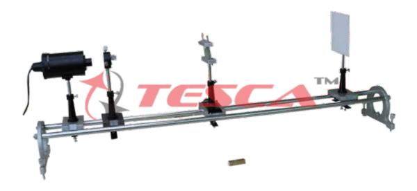
55909 Experimental Set Up has been designed specifically to obtain a lens combination with the specified focal length by using two lenses from the given set of lenses.
