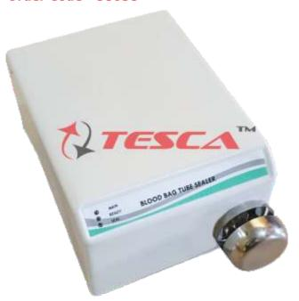
Blood Bag Tube Sealer is a compact equipment to seal the Blood Bag pilot tube by radio frequency sealing system. Sealing can be achieved in less than 1.5 seconds per tube by simple operation. Sealed tube can be easily separated by pulling the sealing section by both sides.
