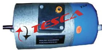
Students can make connections of their own with the help of the terminations provided for study of features viz Starting methods, Speed-Torque, Effect of reduced voltage, Blocked rotor test.
