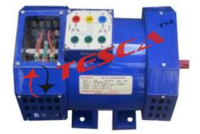
Slipring motor belongs to the family of 3Phase Induction motors, with the difference that the rotor is not same as Induction motors instead has windings with slipring & slipring holder on the rotor. These motors find major application in Crane applications & had the advantage over induction motors that by inserting resistance in the rotor winding the speed can be varied, though this advantage is not valid today as Induction motors have go VVVF drives for speed control.
