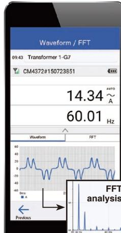
Waveforms such as current and voltage, and FFT analysis waveforms can be displayed.
