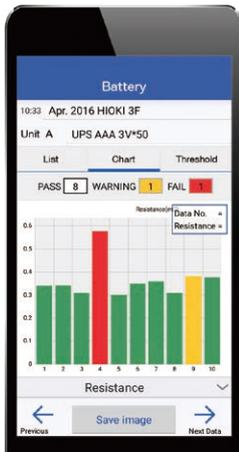
The measured value is compared with the judgment value, and the result is displayed in PASS/WARNING/FAIL.
