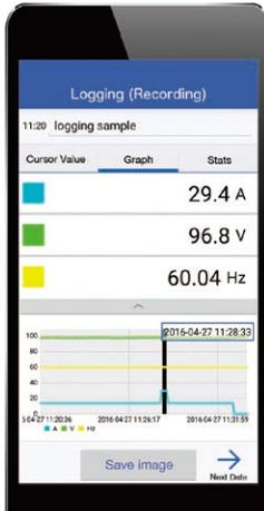
Measurement values can be saved at set recording intervals. You can also check the maximum, minimum, and average values.
