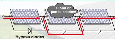
When a solar panel is obscured by a partial shadow (or when it fails), the current bypasses the panel in order to prevent any drop-off in generating efficiency.
