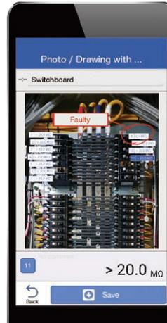
Measurements can be recorded on top of captured photos or imported drawing data.
