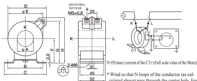
\* Wind so that N loops of the conductor (as calculated above) pass through the center hole. For example, for 120 A:30 A, 4 loops (120 A / 30 A = 4) should pass through the center hole.
