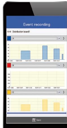
When a value greater than the threshold is measured, the time of occurrence, end time, and the maximum value for that period are recorded.
