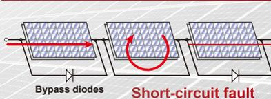
When a short-circuit fault occurs, the generated current flows in a loop, making it impossible to capture the generated power, resulting in lowered efficiency.
