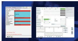
The MD III™ has auto-diagnosis to provide an immediate health status report. Route-based testing and trending features make this an ideal instrument for predictive maintenance. The MD III reports provide an indication of early winding faults, rotor problems, incoming power issues, electrical and mechanical motor condition, and driven load mechanical condition.
