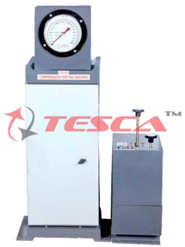
Order Code - MT005 **Compression Testing Machine Analog -**Single Gauge - 1000 KN
