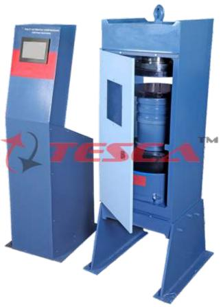
Manufactured as per International design, Plate model for highest mechanical stability, accurate centering of load and excellent repeatability. Fully Automatic pace rate control, auto stop and auto release on failure of test specimen, can be attached with flexural load frame or 500 KN load frame.
