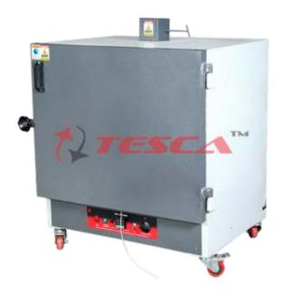
In this system, there is one path of circulating hot air between the inner chamber and insulation. Forced air moved by the motorized blower is called perfect system. It results in minimum temperature variation at any given point in working space.
