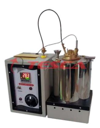
This apparatus is suitable for determining the close cup flash point of petroleum and mixtures according to IP 33 and IP 170 and also IS 1448 (Part I) 1985 (P:20). It is suitable for oils whose flashes below 70°C. It is supplied with oil cup, cover fitted with Geared FHP Motor driven stirrer(120 RPM), thermometer socket, S.S. Water Bath, Stand. An electric heater is fitted at bottom for operation on 220 Volts AC Circuits.
