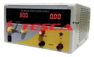
DC Regulated Power Supply is an easy to use, low ripple high regulation precision instrument. It is particularly suitable for experimental development and low voltage applications. Its unique feature is over load protection, which makes it a safe power source for testing of electronic equipment.
