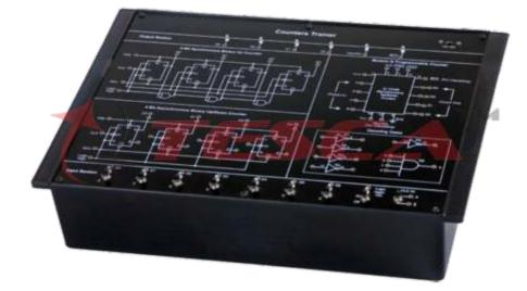
**38717** Counters Trainer is a compact, ready to use digital electronics experiment board. It helps students to get a practical insight into the working of the counters. Counters are undoubtedly the most important part of any digital circuit. Various applications of a Counters include counting events or time periods, dividing frequency, addressing and serving as memory units.
