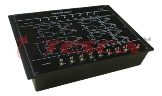
38712 The Flip-Flop Demonstrator is an elite training system for the digital laboratories. It is useful in understanding the working of digital flip-flops.
