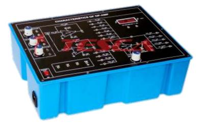
36318 Experimental Training Board has been designed specifically for the study of OP-AMP CHARACTERISTICS ICs 741.
