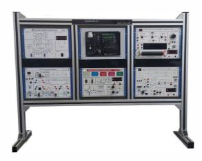
The Sensor Trainer Kit is a modularly designed complete training kit with all the necessary sensors, sources, electronic instrumentation, necessary jigs & displays. Experimentation is down by 2mm brass terminations & patch cords The trainer is housed in an elegant & sturdy plastic cabinets and consists of mimicked dedicated circuits / blocks with necessary test points. The various sensors covered are;
