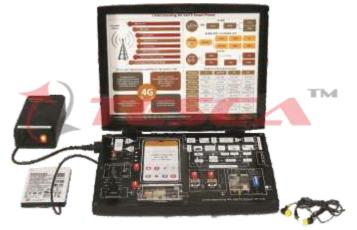
10903D Understanding 4G VoLTE Smart Phone is a unique, self contained, easy to operate, training and platform that demonstrates the complete study and working of a 4G Dual SIM VoLTE handset to understand the fundamentals of Smart phone.
