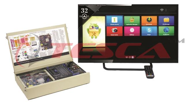
10937B Understanding Wi-Fi / Smart LED Television is a friendly training platform to learn the operation of Wi-Fi/Smart LED Television receiver. It is demonstrator cum training system specifically designed for the comprehensive practical study on Wi-Fi/Smart LED TV engineering for the beginners with a basic knowledge of the various electronic building blocks and fundamentals of communication system.
