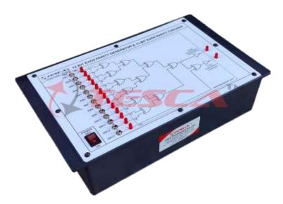
38708 Experimental Training Board has been designed specifically for the study of Even Parity Generator and Even Parity Checker in solid state version. Even Parity Generator and Even Parity Checker play an important role in error detection. As Even Parity Generator and Even Parity Checker are now a days being used quite extensively in electronics, this Training Board has great educational value.
