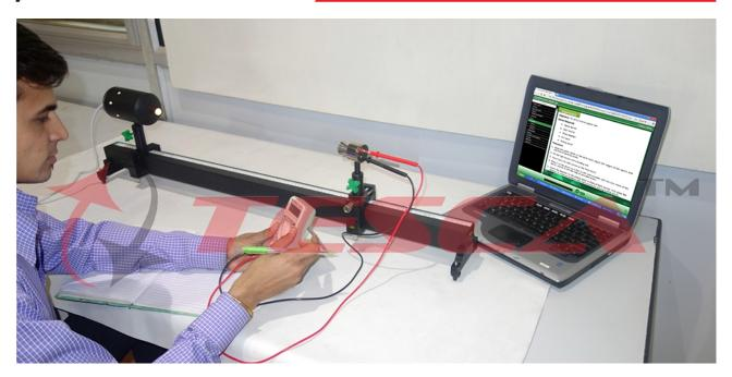
55921B Inverse Square Law Demonstrator is an Optical Setup that describes the variation of light intensity with distance. The Inverse Square Law states that the illumination of a surface by a point source is Inversely proportional to the Square of the distance between the source and surface. Inverse Square Law Demonstrator consists of Optics Bench, Light Source, Photo detector for detecting the Intensity.
