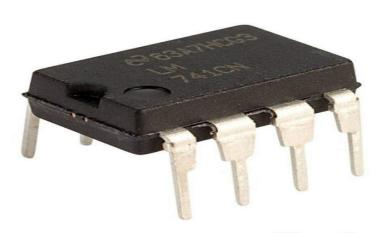
**Technical Specifications:-** The LM741 series are general-purpose operational amplifiers which feature improved performance over industry standards like the LM709. They are direct, plug-in replacements for the 709C, LM201, MC1439, and 748 in most applications. The amplifiers offer many features which make their application nearly foolproof: overload protection on the input and output, no latch-up when the common-mode range is exceeded, as well as freedom from oscillations.
