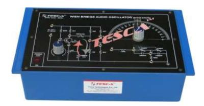
Experimental Training Board has been designed specifically for the study of Wien Bridge Audio Oscillator. This Training Board helps to understand the utilization of Audio Oscillator and obtain oscillations at different frequencies.
