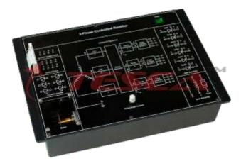
46912 Three phase Controlled Rectifier has been specifically designed to understand the working of Three phase controlled Rectifier with various load configurations. It also helps the students to understand the working of SCR firing fundamentals.
