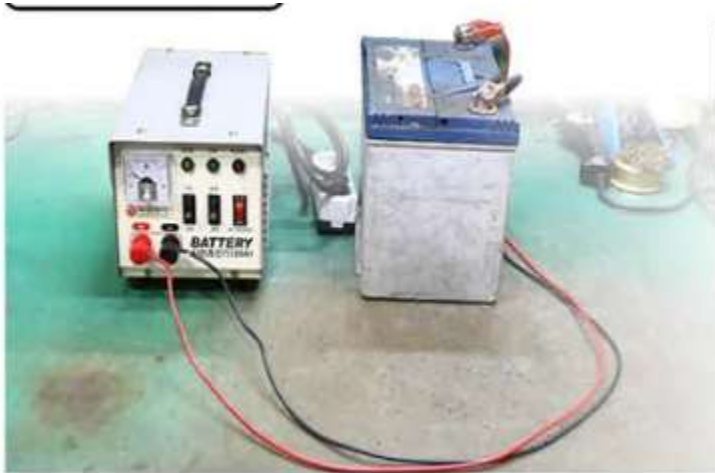
Current meter moves to the right when Charging is in progress and drops to "0" little by little
