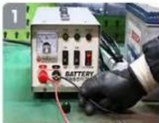
1 Tighten the + red and - black tongs perfectly to the output terminal.
