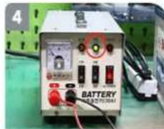
Current meter moves to the right when Charging is in progress and drops to "0" little by little
