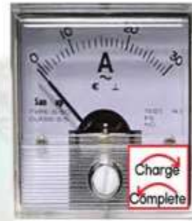
Current meter moves to the right when Charging is in progress and drops to "0" little by little
