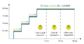
cable insulation. Moreover, a partial discharge measurement shows and locates the PD faults precisely. The highlight of MWT is the condition-based test duration: Provided it is permitted, the test duration can be shortened, which in turn lowers costs. This way, the cable is only exposed to the increased test voltage for the required duration.
