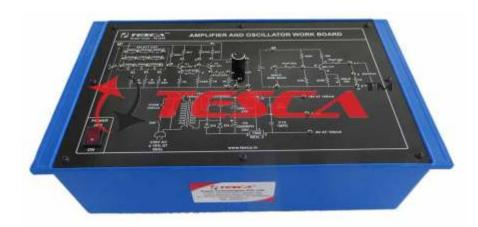
Order Code 36125A Experimental Training Board has been designed specifically for the study of Phase Shift Audio Oscillator & CE amplifier. With the help of this Training Board student can understand the utilization of Audio Oscillator and obtain oscillations of different frequencies with CE amplifier circuit.
