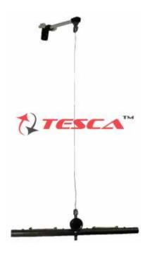
55736 Experimental Set Up has been designed specifically to find the value of modulus of rigidity 'h' of material of the given wire with Maxwell's needle.
