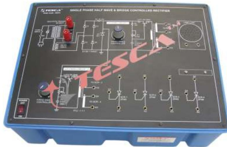
Power Electronic Training Board has been designed specifically to single phase half wave & bridge controlled rectifier.
