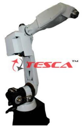
The 54022 is articulated industrial robots are designed to offer customers sturdgy, performance driven robotic solution. 54022 robot is offered with 10 kg payload. Designed and built in India, the robots offer easily accessible automation and productivity solution to customers in micro, small, medium business sectors. • Adaptable to shop floor environment
