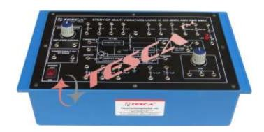
Experimental Training Board has been designed specifically for the study of Bistable, Astable and Monostable Multivibrators using IC 555.
