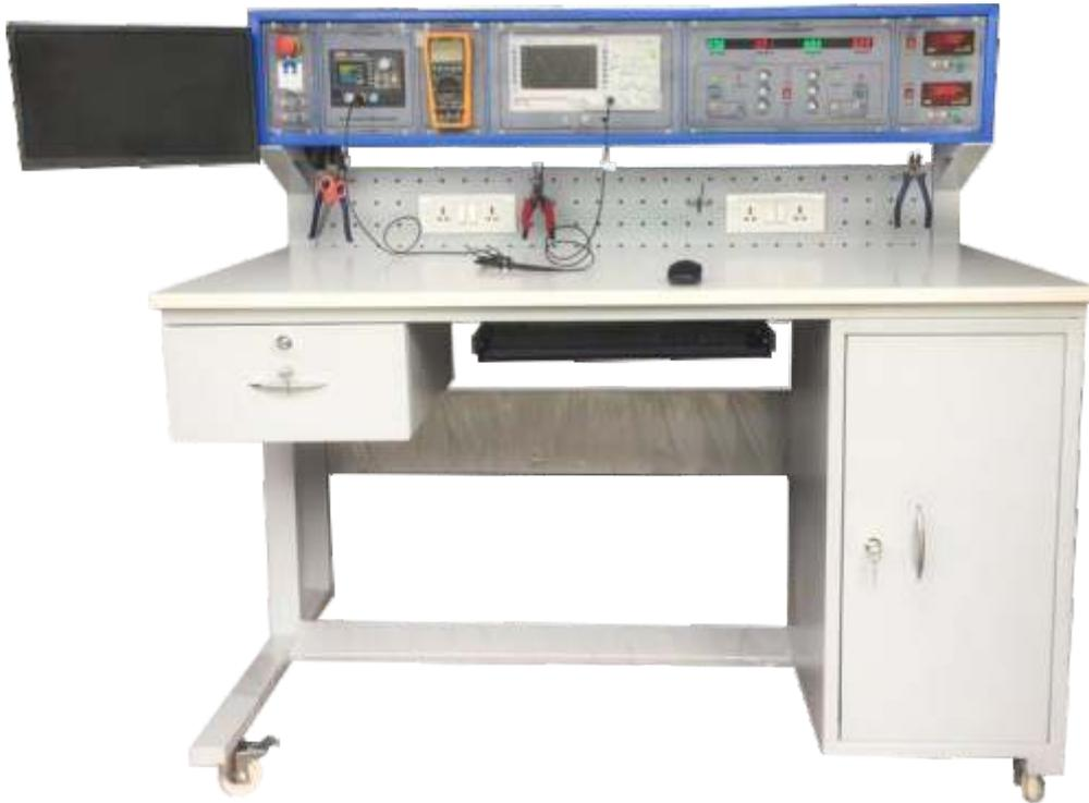
Test Bench for Electrical and Electronics Lab consists of Instruments, panel meters, and required instruments and working area.
