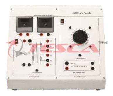
46901 "AC Power Supply" is a versatile product mainly used in electrical and electronic engineering laboratories for the purpose of conducting experiments over AC circuits. This unit provides 0-220V Variable AC output and 6V-0-6V & 12V-0-12V step down AC Voltage with adequate protection schemes. Digital voltmeter and ammeter are being used for better resolution and accuracy.
