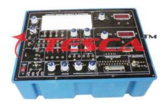
33530 Circuits Development Platform is designed to do experimentation with Analog & Digital Circuits in the laboratory. It is a self contained trainer including DC Power supplies, Sine/Square/TTL Generator etc on as a single unit. It is very useful in project work and testing. A number of ready to use experiment circuit boards are optionally available.
