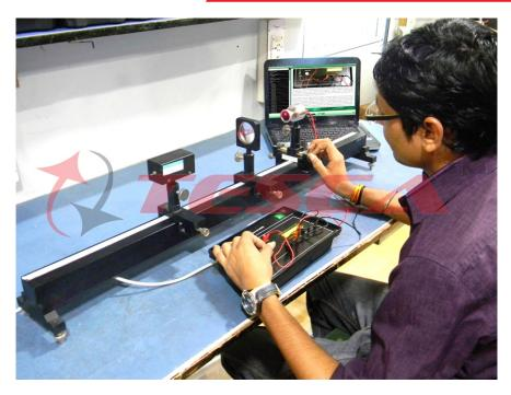
55921A Divergence of LASER is an Optical setup helpful to identify characteristic of LASER beam. This product illustrates how the spreading of LASER beam enhances with respect to distance travelled in a medium. 55921A consists of Optics Bench and Measurement unit. The Measurement unit consists of variable DC power supply, voltage and current display. The Optics Bench consists of LASER source, Converging lens and Photo detector with distance measurement arrangement.
