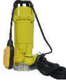
Order Code - TT-WPE-37SB Rated Power: 0.37 kW (0.5 hp) Speed: 2880 RPM Type: 1 Phase Induction Motor Poles: 4; Frequency: 50 Hz Voltage: 220-240V Ampere: 2.86 A Winding: Copper Discharge Range: 20-100 LPM Max Head: 16 m; Min Head: 8m Pump Delivery Size: 25 mm
