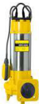
Order Code - TT-WPE-800C Rated Power: 0.8 kW (1.1 hp) Speed: 2850 RPM Max Flow Rate: 300 L/min Max Head: 14 m Electric Source: 220V/50Hz Phase: Single Insulation: B Discharge: 2"
