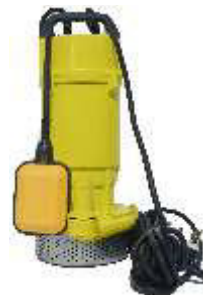
Order Code - TT-WPE-75SB Rated Power: 0.75 kW (1 hp) Speed: 2880 RPM Type: 1 Phase Induction Motor Poles: 4; Frequency: 50 Hz Voltage: 220-240V Ampere: 7.8 A Winding: Copper Discharge Range: 20-133 LPM Max Head: 32m; Min Head: 15m Pump Delivery Size: 25 mm
