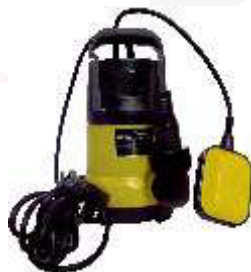
Order Code - TT-WPE-400SB Rated Power: 0.4 kW (0.55 hp) Speed: 2880 RPM Type: 1 Phase Induction Motor Poles: 4; Frequency: 50 Hz Voltage: 220-240V Ampere: 1.75 A Winding: Copper Discharge Range: 15-120 LPM Max Head: 7m; Min Head: 2.3m Pump Delivery Size: 32 mm
