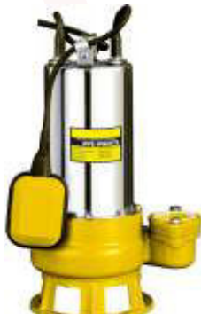
Order Co. - TT-WPE-WQDR15 Rated Power: 1.5 kW (2 hp) Speed: 2850 RPM Max Flow Rate: 800 L/min Max Head: 15 m Electric Source: 220V~50Hz Voltage: 1500 W Insulation: Class B Protection: Ip68
