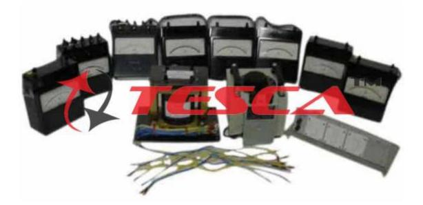
55833 Experimental setup has been designed Specifically to study the performance of transformer and determine open circuit test, short circuit test, efficiency and voltage regulation of 1f Transformer. The setup consist of voltmeters, ammeters, wattmeters, load resistors variac and transformer.
