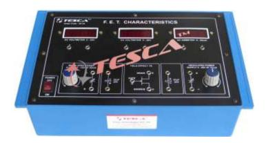
Experimental Training Board has been designed specifically to study the characteristics of a Field Effect Transistor. The board is absolutely self contained and requires no other apparatus.
