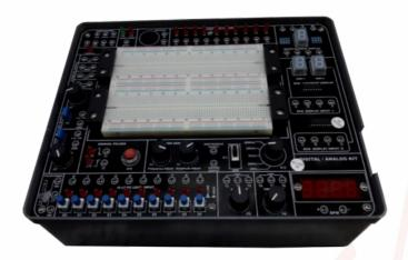
A Single Board Trainer Kit which is widely used to train engineers to Develop/Study hardware for any Digital / Analog components in laboratory. This board has the provision for bread board which facilitates experimenting the **Digital / Analog component Circuits**
