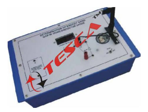
Experimental Training Board has been designed specifically for Determination of Energy Band Gap in Semiconductor (P-N Junction Diode) using Temperature dependent of reverse saturation current. The board is absolutely self contained and requires no other apparatus.
